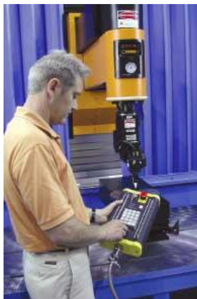
The 790 BeamDirector accepts CO 2 and Nd:YAG lasers for cutting, drilling, and welding 2D and 3D parts.
