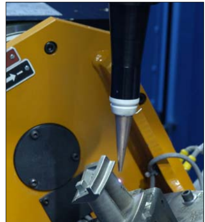
Fig. 4: A laser drilling head fitted with Optical Focus Control. OFC uses a diode laser coaxial with the drilling laser to detect the surface at the drilling location. This approach works with both coated and uncoated surfaces.
