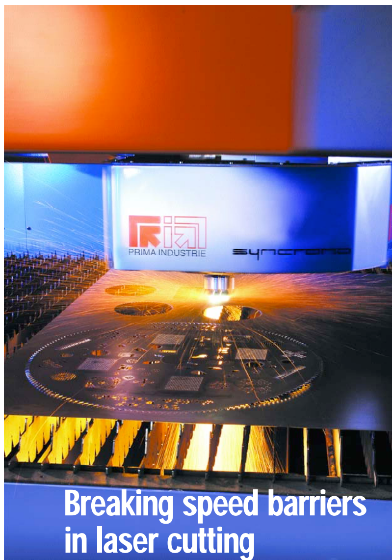
FIGURE 1 Laser cutting devices that have two additional parallel kinematic drive axes on the laser head can cut more than 1,000 holes per minute.
