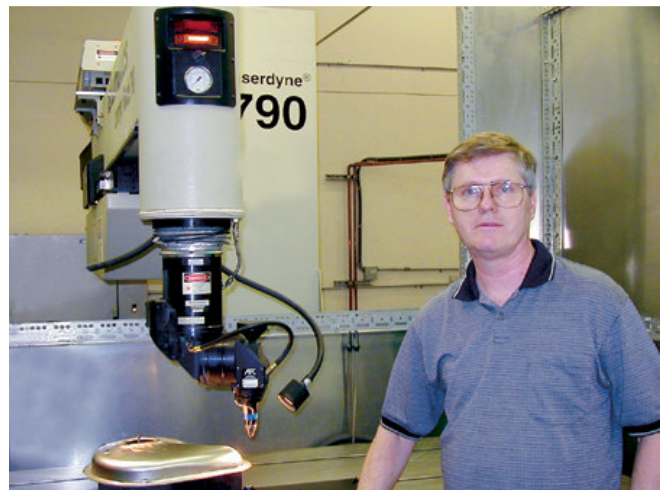
PHOTO ONE CAPTION: Ron Sanders with one of his two Laserdyne 790 BeamDirector Systems. Because the laser moves at all angles to the part, tooling is much simpler and less costly than other types of lasers.
