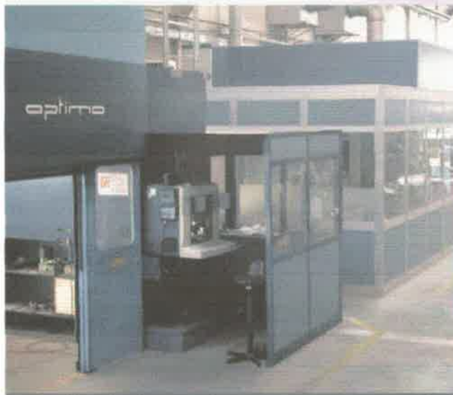
FIGURE 1. The work floor at Sallig includes an installation of four Prima Industrie Optimo laser systems for the processing of prototypes.
