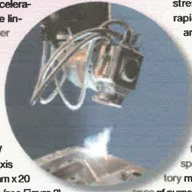
FIGURE 4. Laser welding with the Vivida head from Prima Industrie's Optimo system
