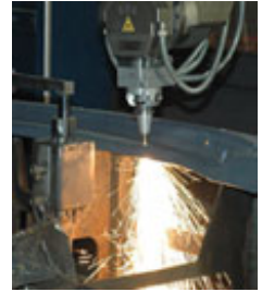
Advanced high-strength steel and ultra high-strength steel parts can be hard to cut—but a laser can handle it.
